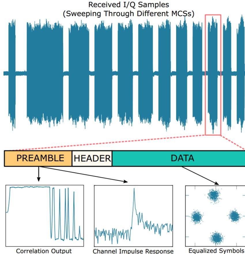
Figure 2: Example of multiple frames with different MCSs captured using *mm-FLEX* (top) and details of different parts of the decoding process (bottom).
