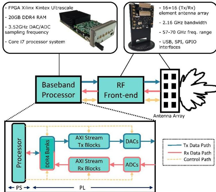
Figure 1: High-level architecture of the platform
