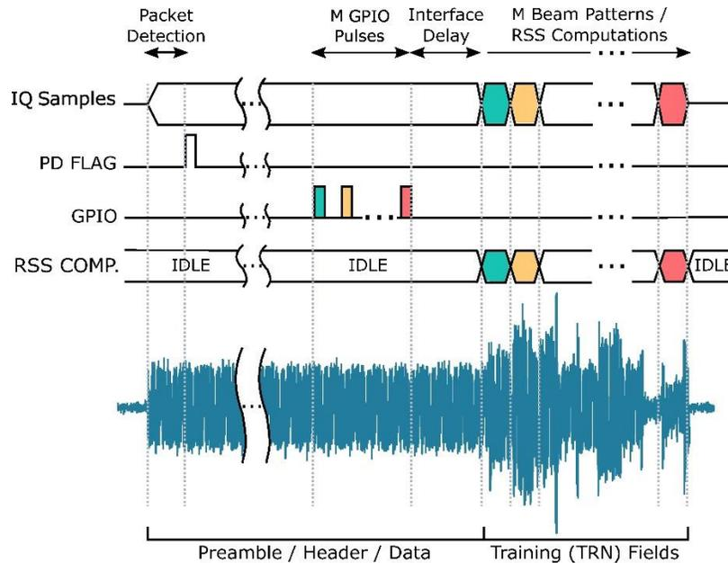
Figure 3: Example of the multiple antenna reconfiguration capabilities of the testbed to implement IEEE 802.11ay *in-packet* training.
