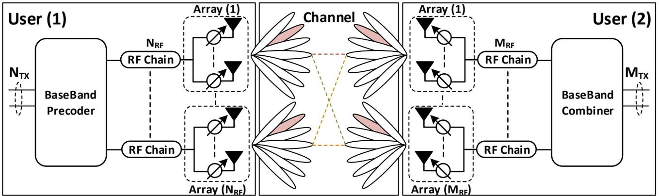
Figure 1: SU-MIMO Partially Connected Beamforming Architecture
