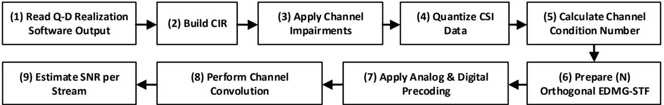
Figure 2: MIMO Simulation Blocks for IEEE 802.11ay in ns-3
