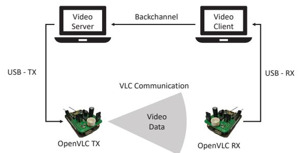
Figure 1: System scheme. Each black line represents a different communication link.
