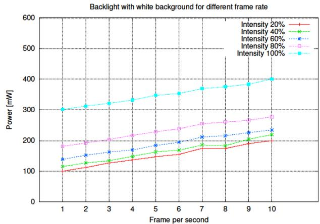
Figure 5: Power consumption of the backlight of a white display for different light levels and screen update speed.
