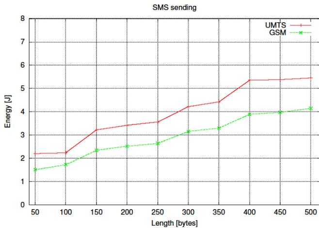
Figure 3: Energy spent for sending text messages with different length.
