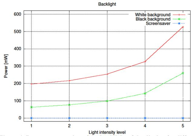
Figure 4: Power consumption of the backlight of the display for different light levels and different background colors.
