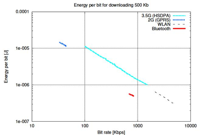
Figure 1: Energy per bit for downloading 500 KB using different wireless technologies.
