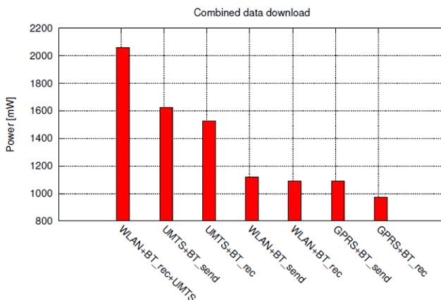
Figure 2: Power consumption for exchange data using different wireless technologies.
