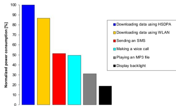
**Figure 6: Top 6 energy consumers on a Nokia N95 mobile phone when switched on.**
