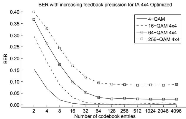
Figure 3: BER with increasing feedback precision for IA.
