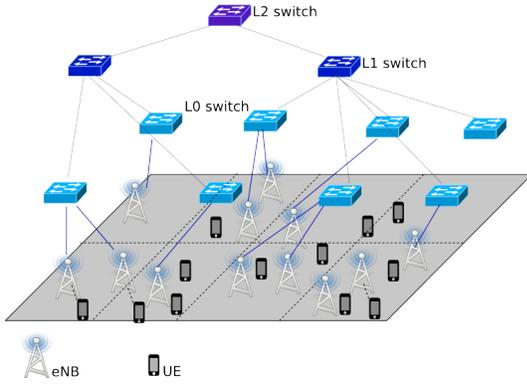
Fig. 1. Example of LTE dense network, with backhaul.
