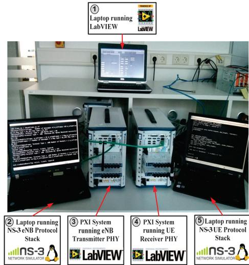
Figure 2: Testbed Setup for eNB-UE downlink scenario.
