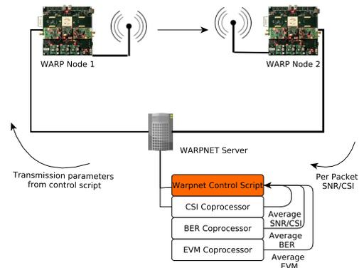
Fig. 2. Experiment setup
