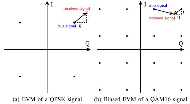
Fig. 1. Example of EVM calculation
