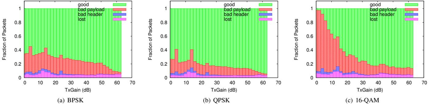
Fig. 3. Packet reception statistic for different modulation schemes
