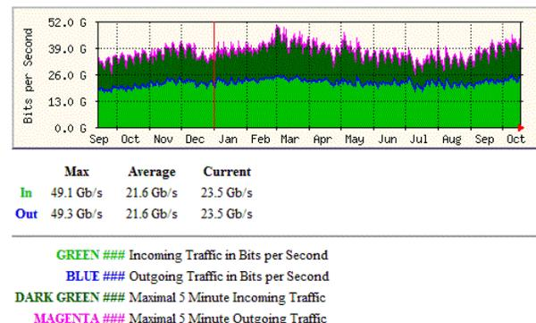
Figure 1: mrtg output for aggregated SIX traffic.
