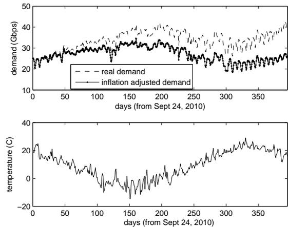
Figure 7: The real and inflation adjusted demand at TORIX (top). Average daily temperature at Toronto (bottom).
