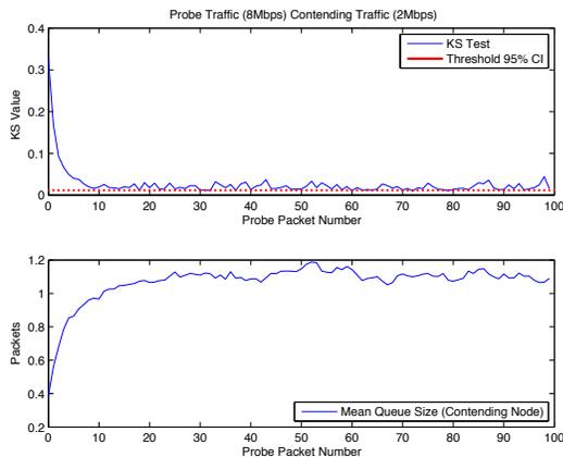
**Figure 8: Analysis of the distribution (8Mbps probe-traffic rate, 2Mbps cross-traffic rate (Top) KS-Test (Bottom) Mean queue size (simulator)**
