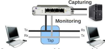
Fig. 1: Measurement architecture with passive tap.
