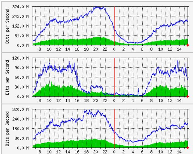
**Figure 1: Demand statistics for partners  $P_1$  (top),  $P_2$  (middle), and  $P_3$  (bottom) in the motivating example: the x-axes are in hours; the y-axes are in  $Mbps$ ; the filled (green) areas depict the upstream traffic; the (blue) lines represent the downstream traffic.**
