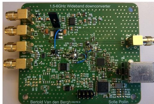
Figure 1. Prototype of the down-converter board
