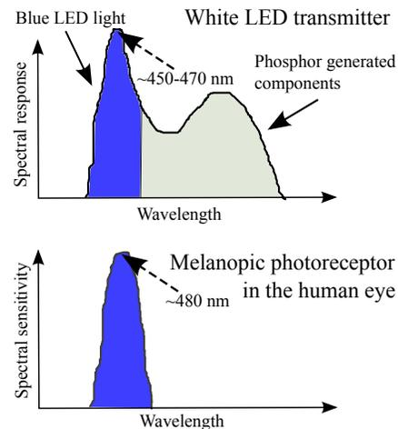
**Figure 1: Top: LED spectrum, blue light components and phosphor-generated components. Bottom: spectral sensitivity of melanopic photoreceptor in the human eye.**
