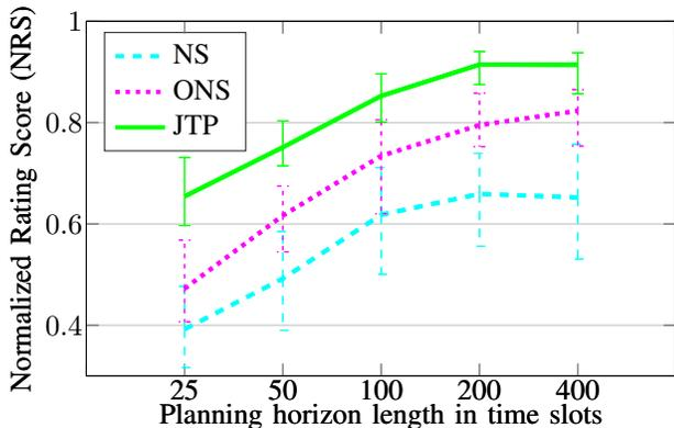
Fig. 1. Normalized Rating Score (NRS) of the transmission planners for different planning time horizon lengths
