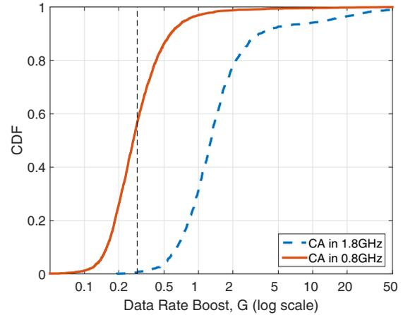
Fig. 4: Data rate increase due to carrier aggregation. The vertical dashed line marks the start of the energetically efficient operations.
