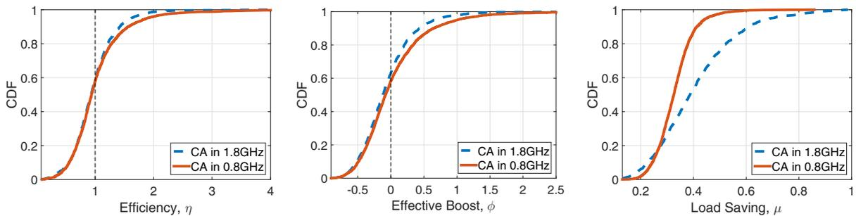
Fig. 5: Comparison of the CA efficiency for 800 MHz and 1800 MHz SCells.
