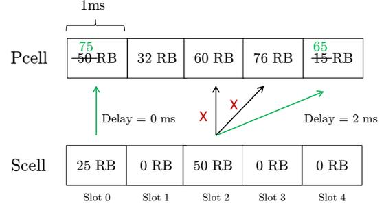
Fig. 2: Delay example for 20MHz band in PCell
