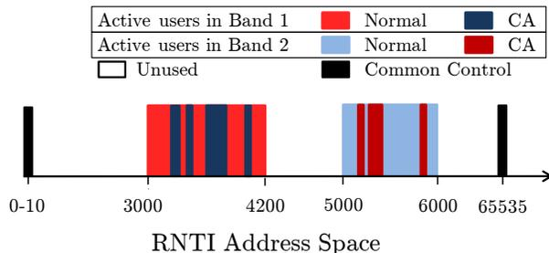
Fig. 1: RNTI utilization for two LTE bands performing carrier aggregation.
