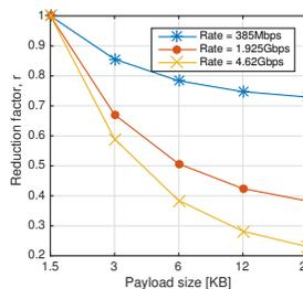
Fig. 4. Collision reduction factor  $r$  for different aggregation levels.
