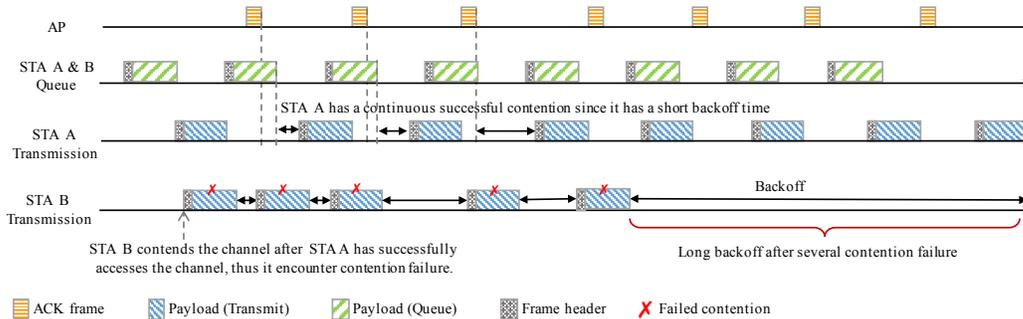
Fig. 2. Channel access frequency for bursty traffic with deaf stations.
