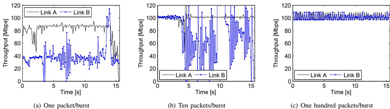
Fig. 8. Throughput of Links A and B for different aggregation levels
