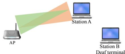
Fig. 1. Station B fails to overhear the transmission between Station A and the AP as it is not within the beam angle of Station A nor the AP.
