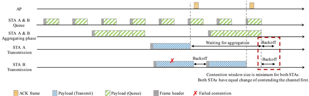
Fig. 3. Aggregation algorithm.
