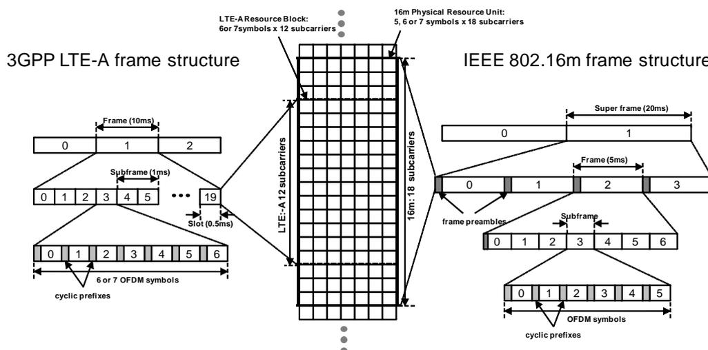
Figure 1: Comparison of LTE-A and IEEE 802.16m frame structure
