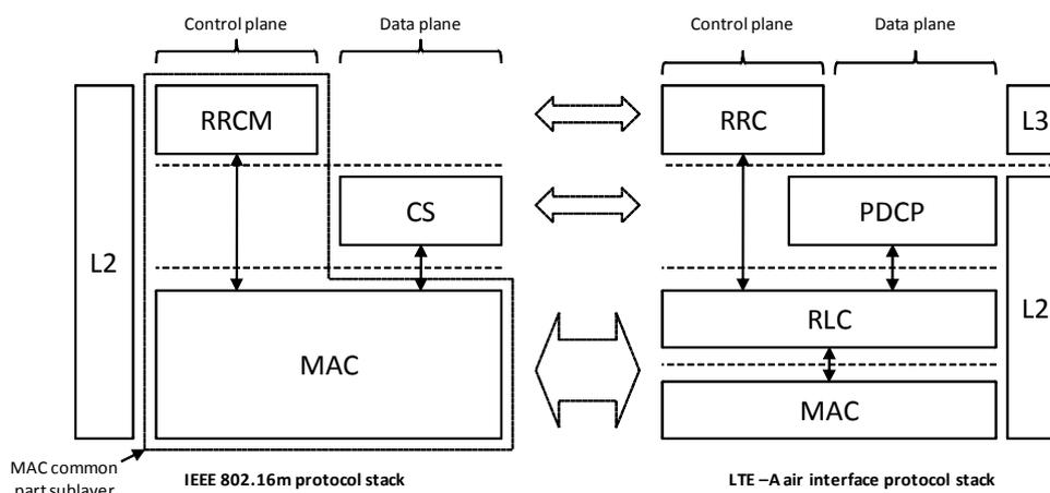
Figure 2: comparison of LTE-A and IEEE 802.16m protocol stack
