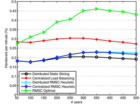
Fig. 4. Average number of handovers per minute per UE for  $T_{Util/Sector} = 10 UEs$
